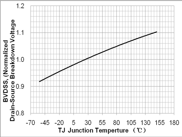
Fig 5. Breakdown Voltage Variation vs. Junction Temperature
